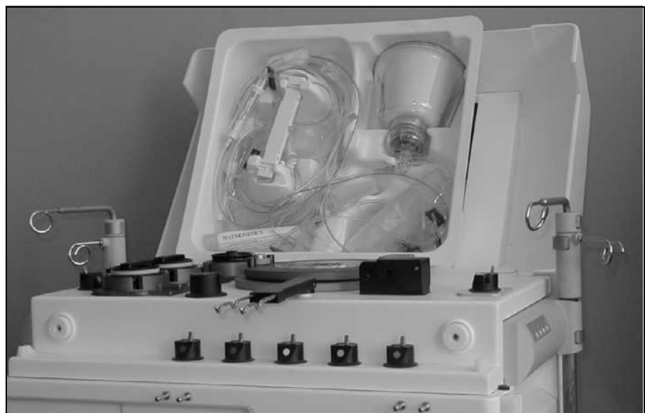
Figure 4-2, The MCS+ disposable set tub is tailored for practical installation
