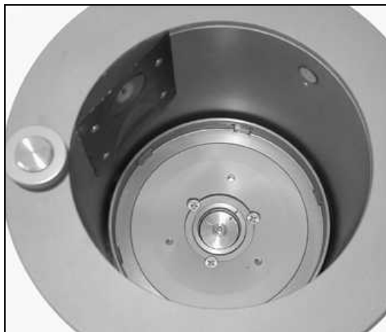
Figure 1-4, MCS+ vacuum centrifuge retrofitted with the mechanical chuck
