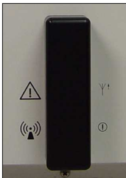
Figure 2-13, Example of the wireless antenna located on the device rear panel
