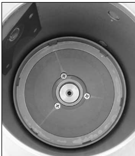
Figure 1-2, MCS+ mechanical centrifuge chuck
