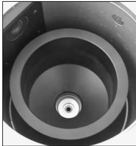
Figure 1-5, MCS+ centrifuge with chuck adapter for blow molded bowl
