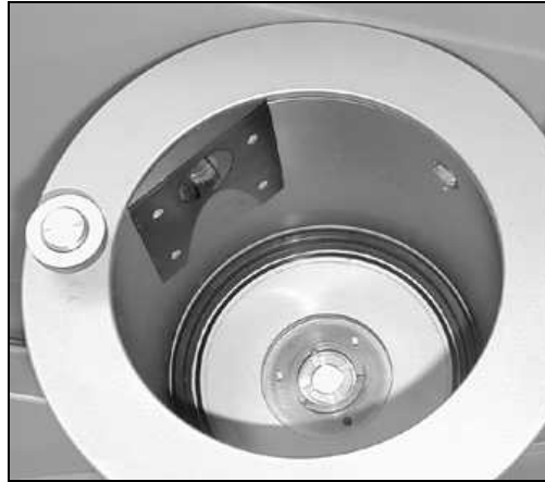
Figure 1-3, MCS+ vacuum centrifuge chuck
