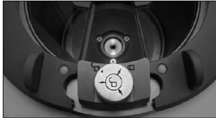
Figure 1-9, Locking knob "PUSH TO OPEN", symbol version
