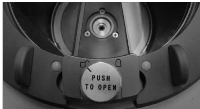
Figure 1-10, Locking knob "PUSH TO OPEN", text version
