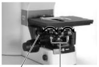
Focus the condenser using the condenser focus knob.
