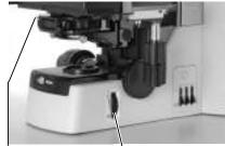
Aperture diaphragm Field diaphragm knob lever
