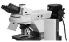
Light shield attached (with Epi-illumination attachment)
