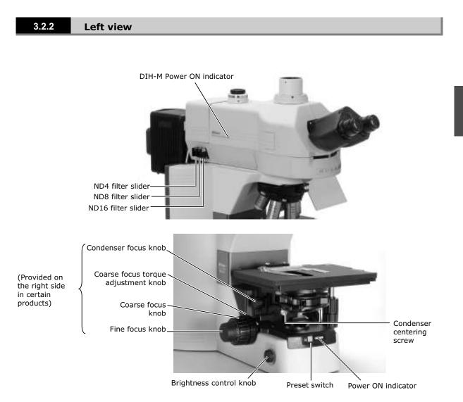
3.2 Names of Parts Used to Make Adjustments
