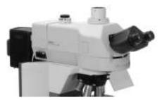
Light shield attached (with DIH-M)
