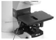
Fixing the stage with centering function
