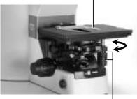
Move the portion to be viewed into the optical path using the XY stage knobs.
