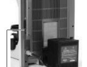
Attach the hand switch for the Epi-illumination shutter here.
