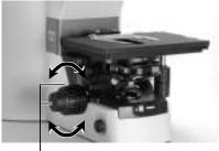
Focus on the specimen using the coarse and fine focus knobs.
