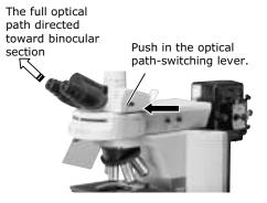
**5** Rotate the excitation method switchover turret to set it at position where no filter cube is installed.
