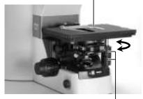
Move the portion to be viewed into the optical path using the XY stage knobs.
