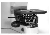
Focus the condenser using the condenser focus knob.
