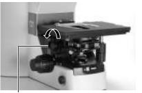
Raise the condenser using the condenser focus knob.
