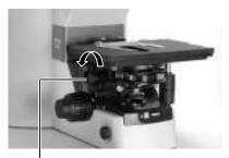
Raise the condenser using the condenser focus knob.
