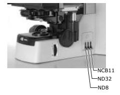
**4** Pull out both optical path switching levers and direct the full optical path toward the binocular section. The full optical path directed toward the binocular section
