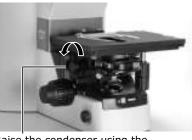
Raise the condenser using the condenser focus knob.
