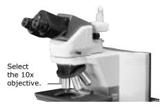
8 Set a specimen and move the portion to be viewed into the optical path.
