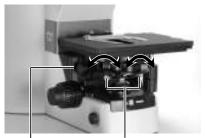
Focus the condenser using the condenser focus knob. Center the condenser using the condenser centering screws.
