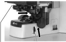
Fully open the aperture Fully open the field diaphragm using the aperture diaphragm lever.
