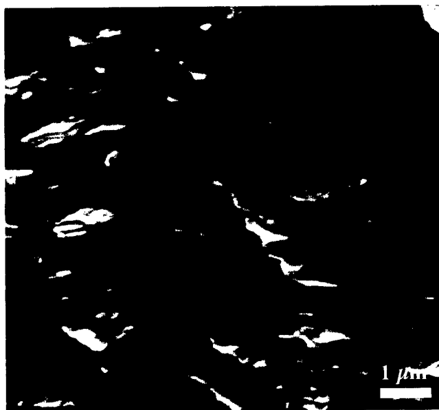
Figure 4.9: Higher magnification view of the untreated surface showing bent basal surfaces
