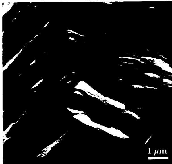
Figure 4.10: Higher magnification view of 15 minute etched surface illustrating the sharp peak-like features on the surface
