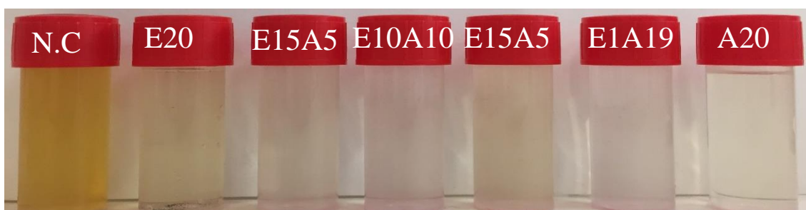
Figure 21. Reaction medium recovered after at the end of the biphasic CWPO runs, upon removal of the catalysts N.C; E20; E15A5; E10A10; E5A15; E1A19; A20, respectively.
