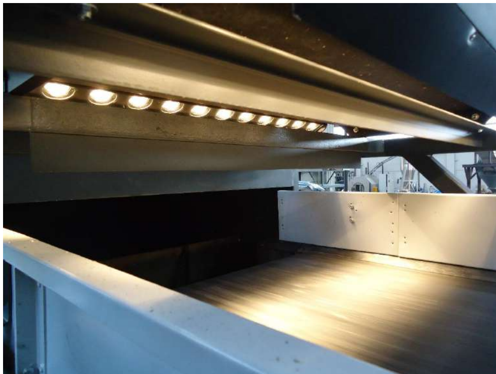
Figure 10 NIR sorting belt showing the lamps emitting the infrared light
