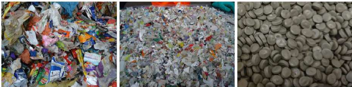
Figure 11 Pilot trial for recycling of a PE/PP mix. Mixed film (left), washed and shredded film (middle) and extruded pellet (right)
