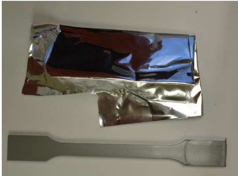
Figure 5 Injection moulded test piece made from metallised PP film
