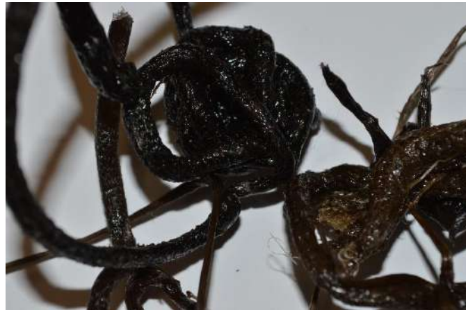
Figure 8 PVdC degradation from extrusion process
