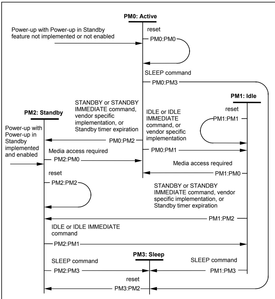
Figure 3 – Power management state diagram
