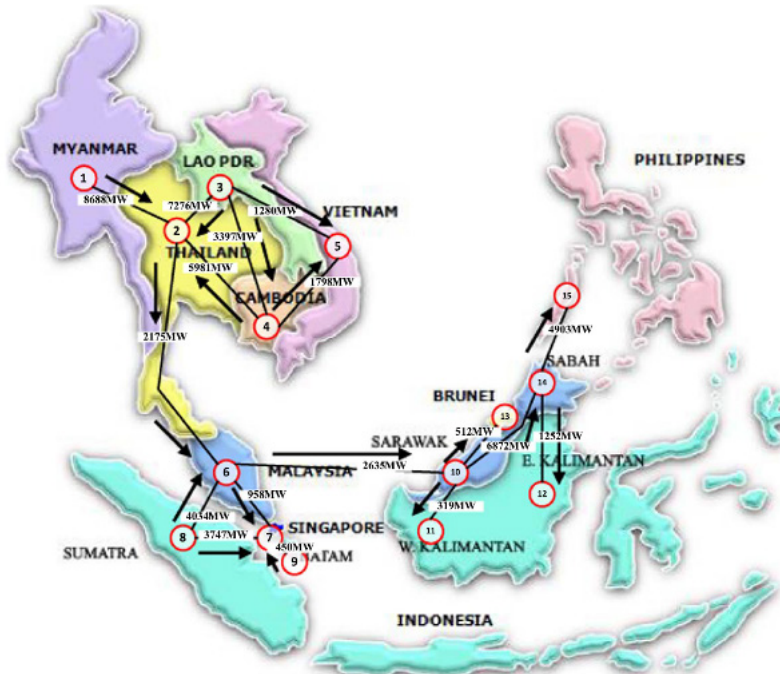
*Numbers in MW and arrows show the maximum power flow between the interconnections and dominant directions Figure 35: Optimal cross-border transmission capacities for ASEAN region in 2030 [199] (used with permission)
