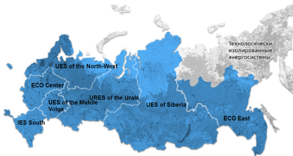
Figure 38: Unified Energy System of Russia (UES of Russia) composed of 7 united energy systems [213]
