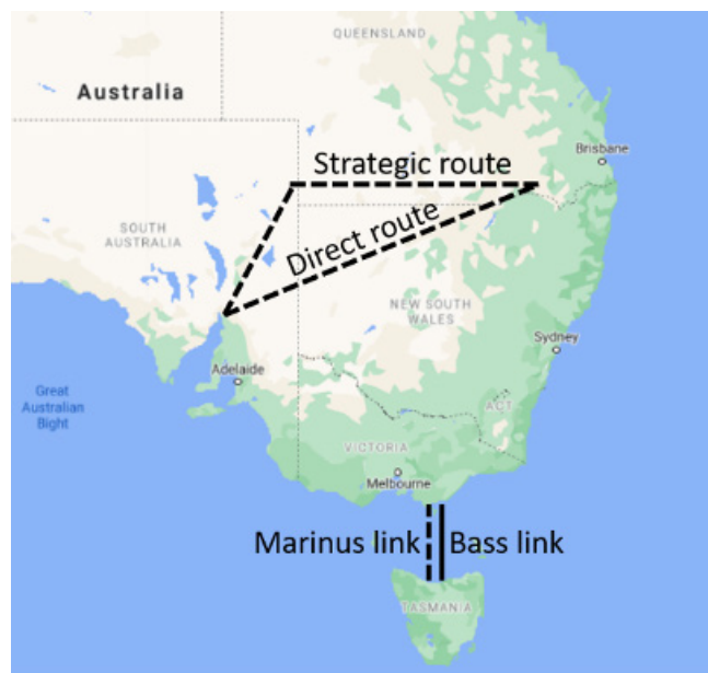
Figure 37: Marinus link and proposed routes for the Trans-Australian HVDC interconnector [adapted from 204]
