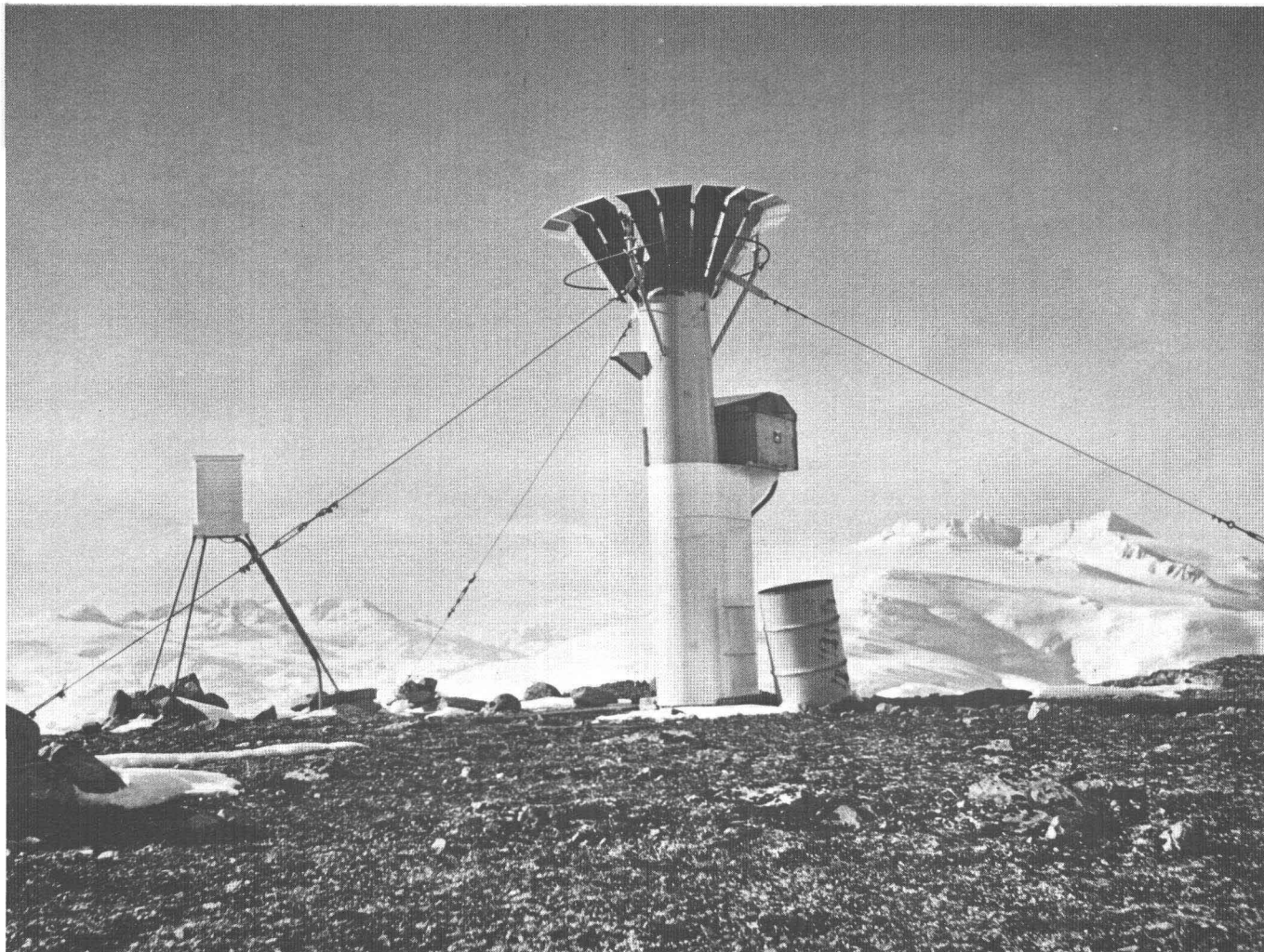
FIGURE 5.—Photograph of precipitation and air-temperature gage at Wolverine Glacier, Kenai Mountains, Alaska. This recording gage operates throughout the year at site 3, 1,000-m altitude (see pl. 3A for location). A specially designed antifreeze solution which is self-mixing enables precipitation occurring as snow to be recorded without the addition of heat. The wind screen on the left contains the air temperature sensing element.
