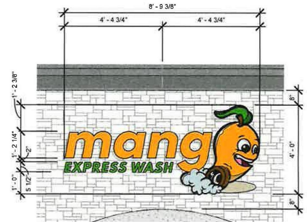
4 BUILDING SIGN (Over Tunnel Doors) SCALE: 3/8" = 1'-0"
