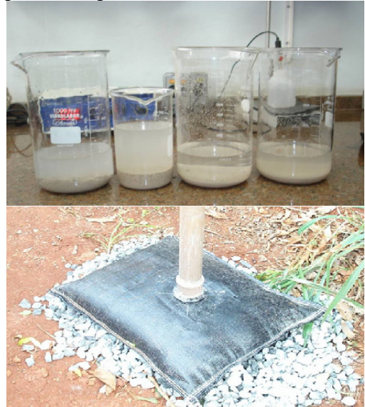
Figure 3.22. Dewatering geotube evaluation: chemical and geotube model tests (Bittar et al., 2010)
