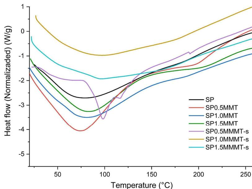
**Figure 7.** DSC thermograms of bionanocomposite films at different concentrations of clay and ultrasound treatment.
