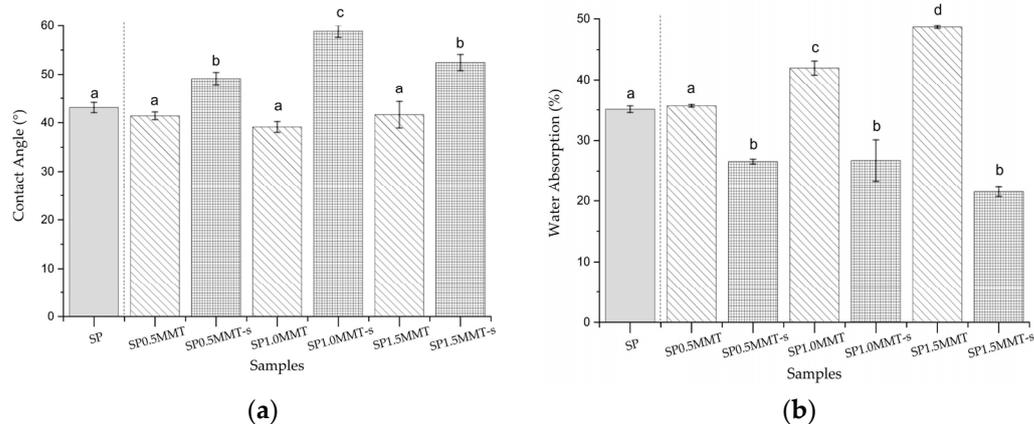
**Figure 8.** Effect of MMT nanoclay concentration and ultrasound treatment on (a) contact angle and (b) water absorption of starch/PVA (SP) composite films. SP control sample without nanoclay. Different letters (a, b, c, d) in the same column denote significant differences for the set of means in each treatment (with and without ultrasound) ( $p < 0.05$ ).
