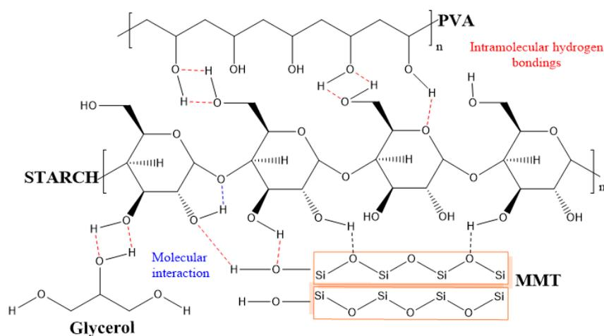
**Figure 5.** Schematic illustration of proposed molecular interactions between polymers (starch and PVA), plasticizer (glycerol), and MMT nanoclay.
