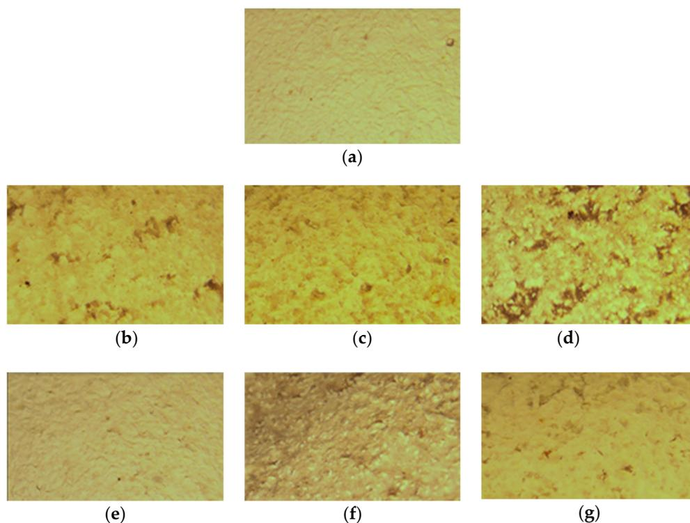
**Figure 1.** Optical microscopy images for (a) achira starch-PVA (SP) films with different concentrations of MMT (0.5, 1.0 and 1.5%), treated with (-s) and without sonication. 10× magnification. (a) SP, (b) SP0.5MMT, (c) SP1.0MMT, (d) SP1.5MMT, (e) SP0.5MMT-s, (f) SP1.0MMT-s, and (g) SP1.5MMT-s.
