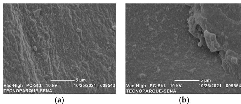
**Figure 3.** SEM micrographs for biodegradable films with MMT nanoclay at 5000× magnification. (a) SP1.5MMT and (b) SP1.5MMT-s.
