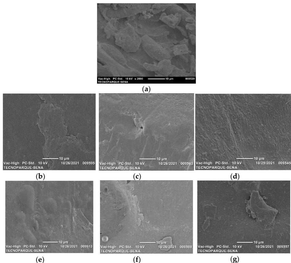
**Figure 2.** SEM micrographs for achira starch-PVA biodegradable films with MMT nanoclay (0.5, 1.0 and 1.5%), treated with (-s) and without sonication. (a) SP, (b) SP0.5MMT, (c) SP1.0MMT, (d) SP1.5MMT, (e) SP0.5MMT-s, (f) SP1.0MMT-s, and (g) SP1.5MMT-s. 2000× magnification.
