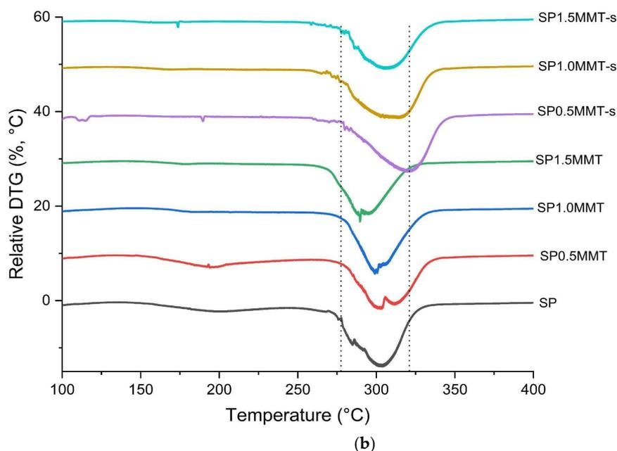
**Figure 6.** Thermogravimetric Analysis (TGA) (a) and Derivative Thermogravimetry (DTG) (b) curves of bionanocomposite films at different concentrations of clay and ultrasound treatment.
