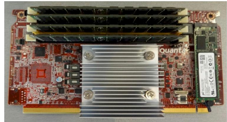
intel created with Xeon D processor and worked with Quanta to design the board and to get the microserver manufactured.
