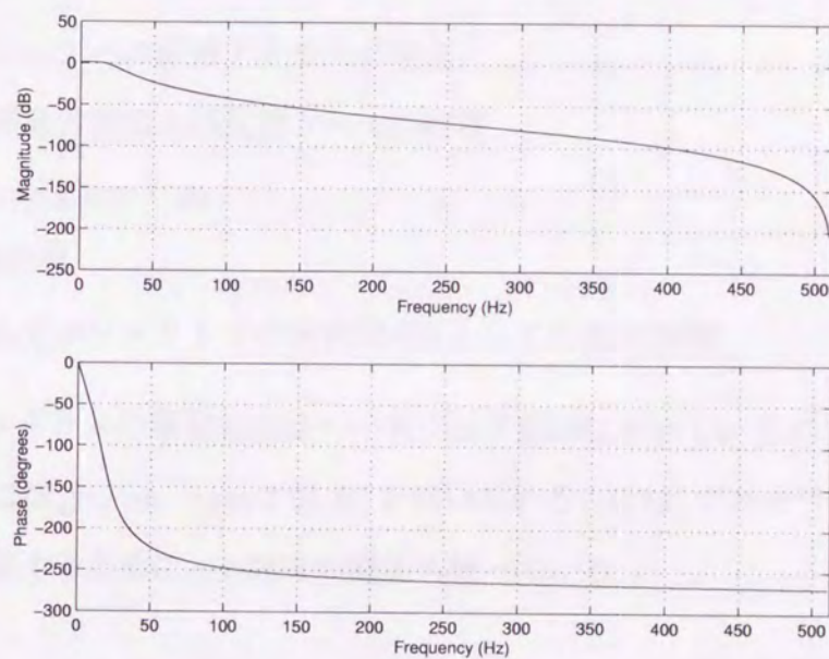
Fig A.14: Bode diagram of butterworth filter
