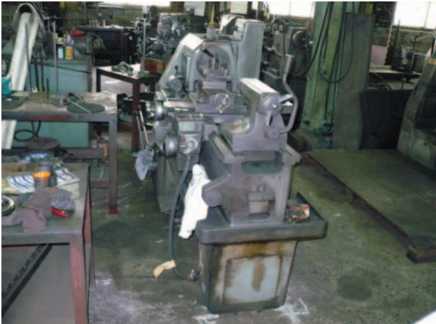
Fig. 4 A small size lathe without anchor bolts which toppled as the earthquake attacked. The photo shows the state after it was raised up and checked horizontal alignment.
