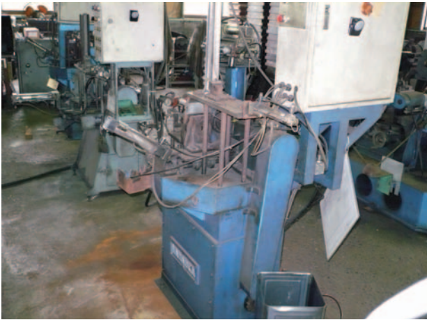
Fig. 5 A special tooling machine whose mounting bracket of pneumatic cylinder deformed when it fell over.
