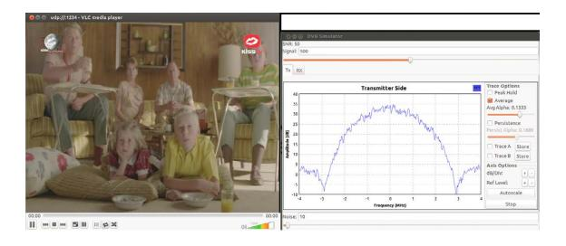
Figure 4.4.6 Video transmission when SNR=50
