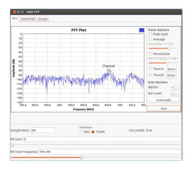
Figure 4.1.3 GSM Channel bump
