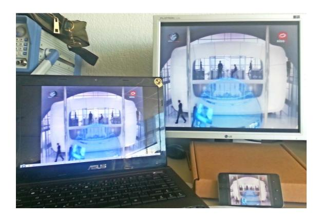
Figure 4.4.7 Broadcasting video on three different clients
