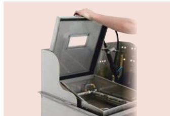
Washing shower equipped with automatic shutoff function, when opened
