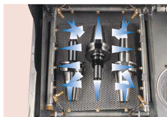
Automatic washing from 18 nozzles.
