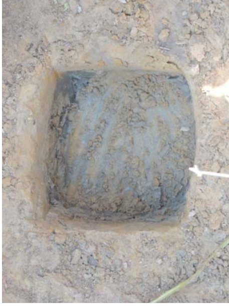
Figure 13. Detail of permeability test hole
