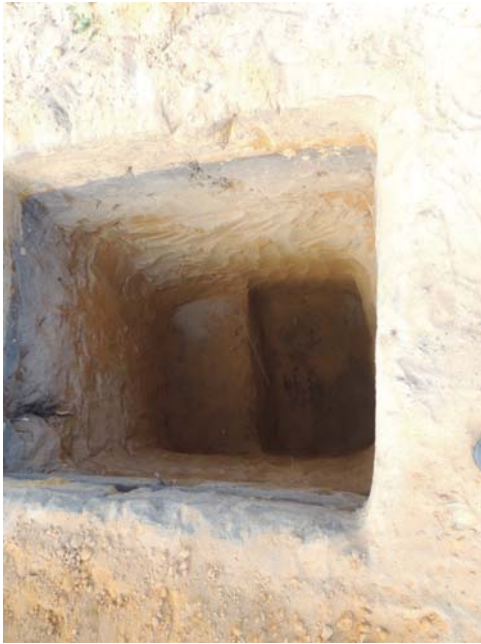
Figure 13. Detail of the Trial Pit showing the oxidized upper layer
