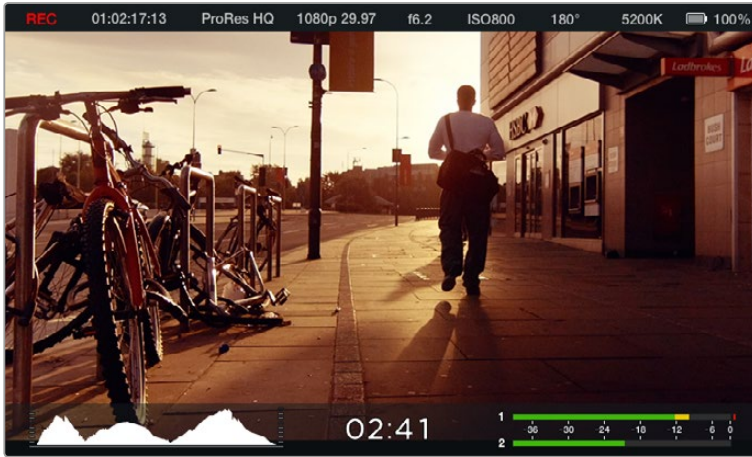
On screen meters and status strip on the Blackmagic Micro Cinema Camera
