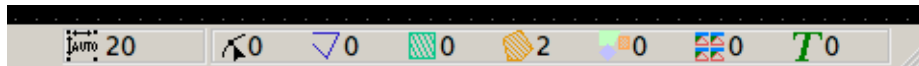
Figure 3.2: The Select Indicator toolbar (lower right corner of the LE window). Two polygons are selected. The spacing between grid points is 20 \mu\text{m} .
