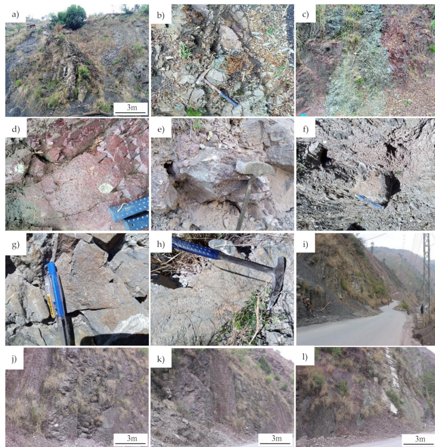
Figure 3. Photomicrograph showing (a) mudstone, (b,l) pencil-like shales, (c) variegated color shale, (d) reduction spots, (e) fine and coarse grain sandstone, (f,g) lenses of limestone, (h) coarse-grained sandstone, (i) lower contact of Kuldana Formation, (j) cyclic deposition of shales and sandstone, (k) sandstone lens in shales, (l) variegated colored pencil-like shales and limestone bed.
