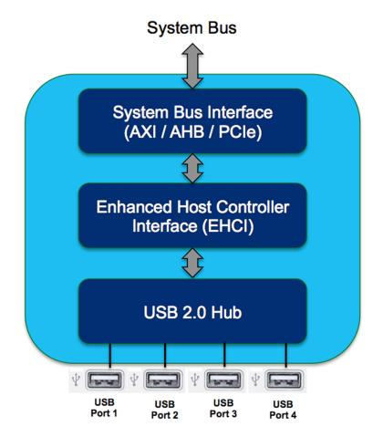
Figure 3: Arasan USB 2.0 Host Controller Solution
