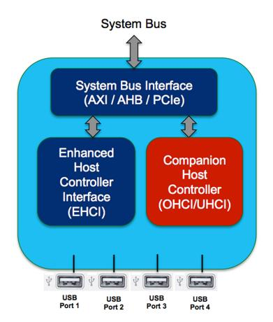
Figure 2: USB 2.0 Host controller with companion host controller
