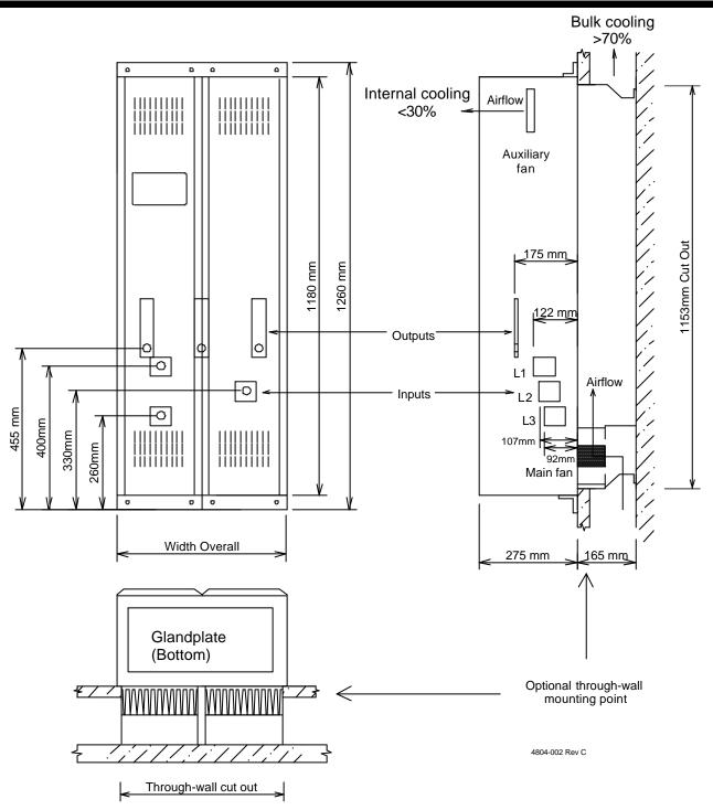
Figure 1.4: Dimensional Details - Microdrive V 170-900A Series.
