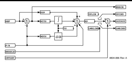
Figure 4.3: PID Controller special function module
