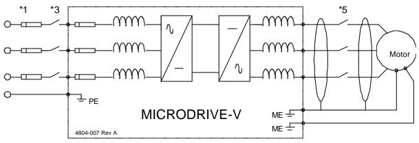
Figure 3.1: Power Connection Details
