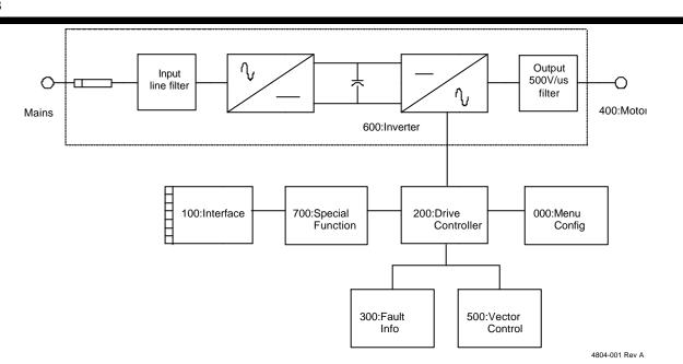
Figure 2.3: Microdrive V Series Block Diagram
