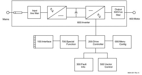
Figure 1.1: Microdrive V Series Block Diagram
