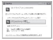
When the setup screen of L-02C connection software is not automatically displayed, install via the included CD-ROM. (→P38) Select "L-02C 接続ソフト、L-02C 接続先(APN) 設定ツール、通信設定ファイル(ドライバ)をインス トールする(推奨) (L-02C connection software, L-02C APN setting tool, Communication configuration file (driver) (recommended))" and click "次へ(Next)"
