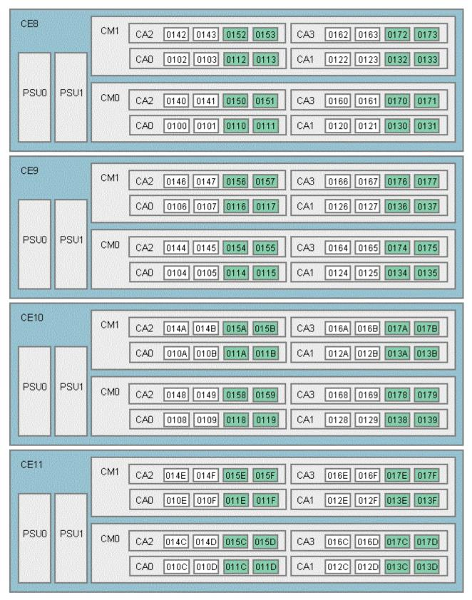
CM: Controller Module, CA: Channel Adapter, PSU: Power Supply Unit
