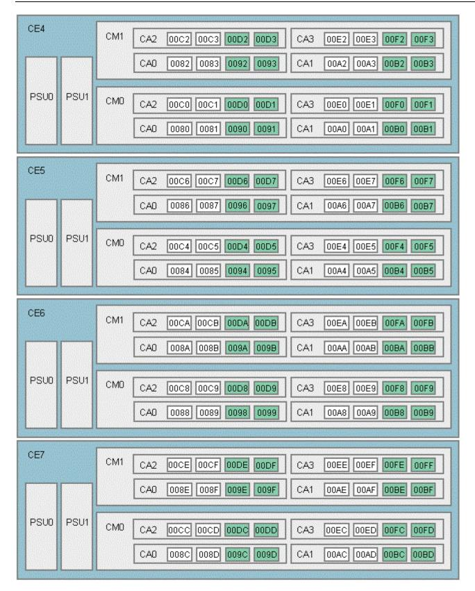
CM: Controller Module, CA: Channel Adapter, PSU: Power Supply Unit
