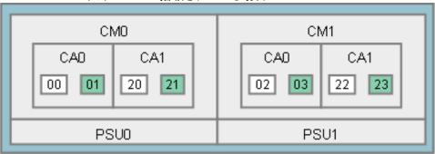
CM: Controller Module, CA: Channel Adapter, PSU: Power Supply Unit
