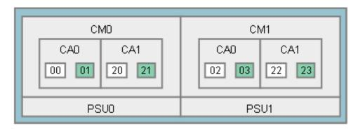
CM: Controller Module, CA: Channel Adapter, PSU: Power Supply Unit
