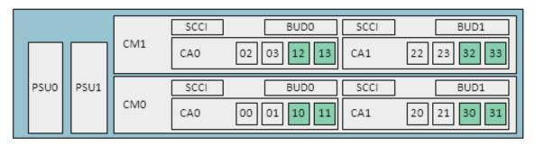
CM: Controller Module, CA: Channel Adapter, PSU: Power Supply Unit
