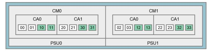
CM: Controller Module, CA: Channel Adapter, PSU: Power Supply Unit
