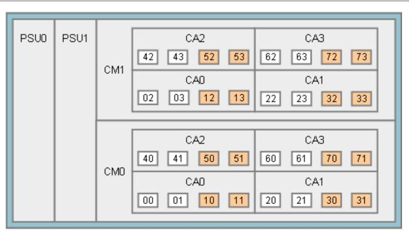
CM: Controller Module, CA: Channel Adapter, PSU: Power Supply Unit
