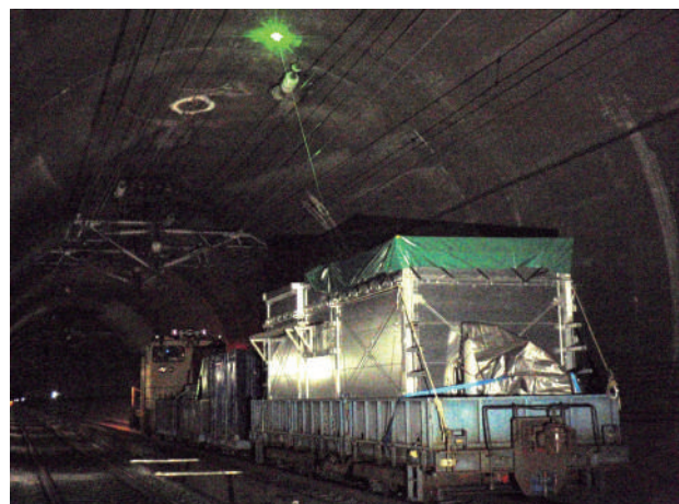
Fig.9 Mobile prototype of laser-based system in operation
