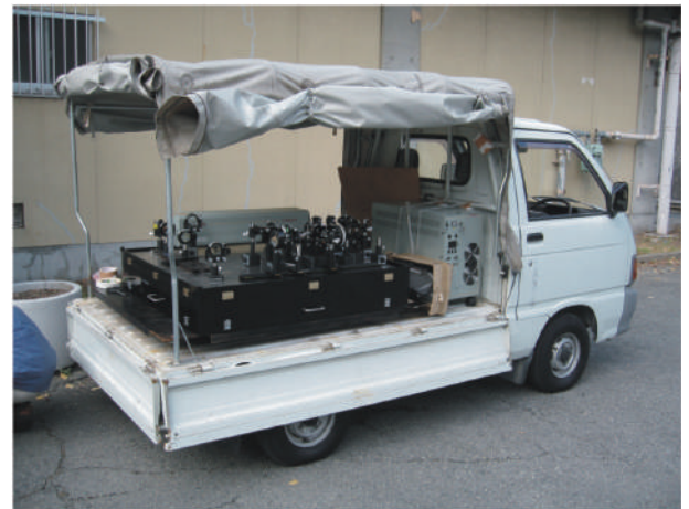
Fig.7 The first mobile prototype of the inspection system
