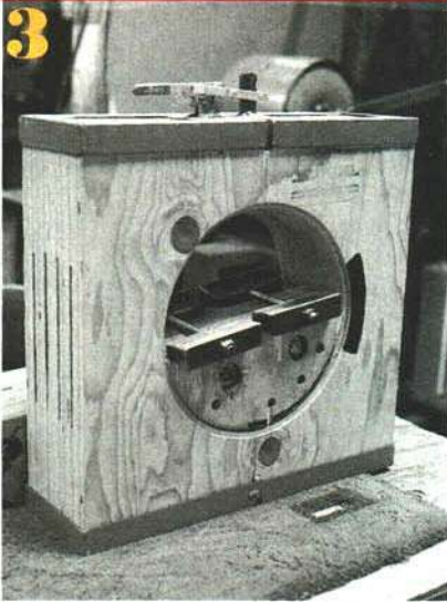
The rolled board is placed in a wooden mold.
