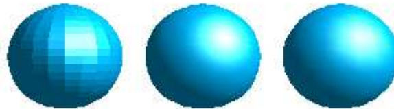
Figure 31 - Shading examples. From left to right: Flat, Phong, Gouraud.
