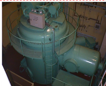
Electron accelerator (0.5~2.0 MeV, 0.1~30 mA)
