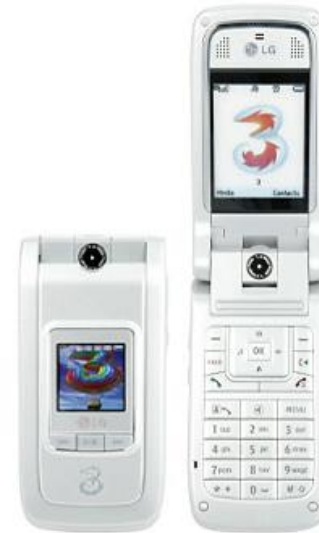
LGE U880 (MSM6250) 2" Mobile XGA Display (220x176) 1.3 MP camera
