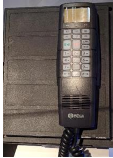
Qualcomm Beta phone Single-chip CDMA MSM in .8\mu process
