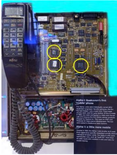
Qualcomm Alpha II phone 3 chip CDMA chipset in 1.2\mu process
