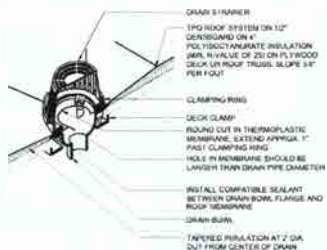
04 ROOF DRAIN DETAIL SCALE: NTS
