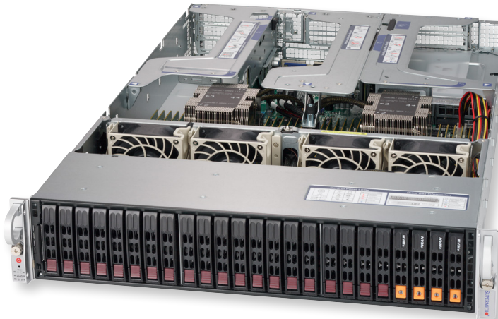
Dual-socket support up to 56 cores / 112 threads
