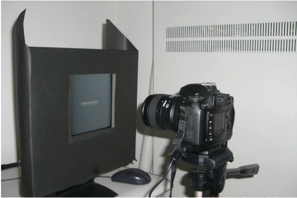
Fig. 6 Geometry of MTF measurement
