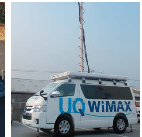
UQ車載基地局 UQ vehicle-mounted mobile base station
