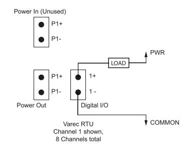
Figure 6-8: 8813 DC Output Wiring Diagram
