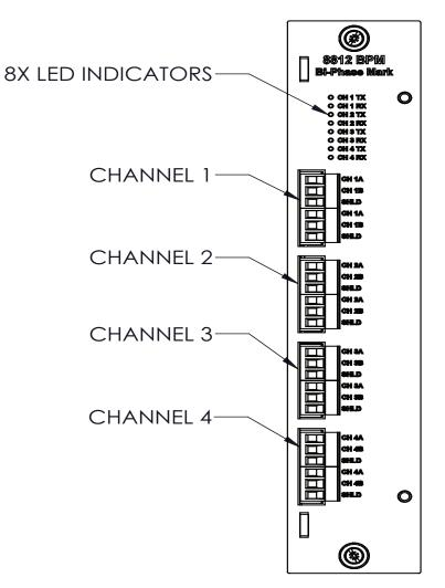
Figure 5–2: 8812 Bi–Phase Mark Module Face Plate
