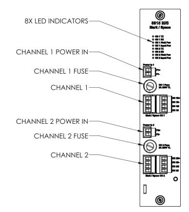
*Figure 8–1: 8815 Varec Mark/Space Interface Module*
