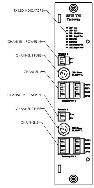
Figure 9–1: 8816 TW Tankway Module Face Plate
