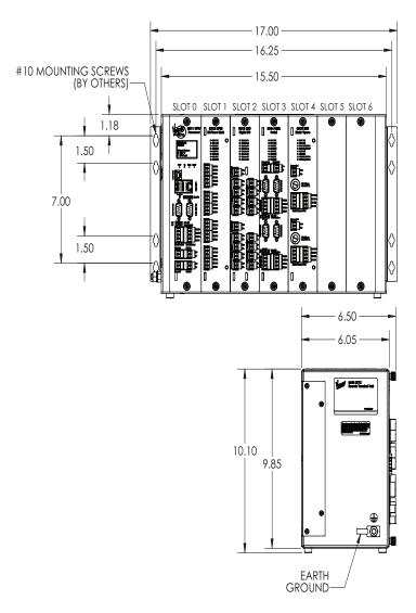
Figure 3-2: 8810 RTU Dimension Drawing
