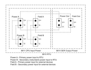
Figure 4-4: RTU Internal Power Circuitry
