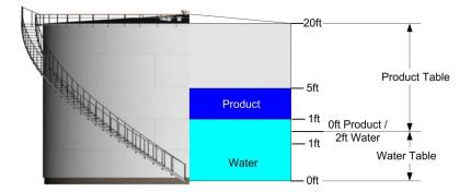
Example 2 shows how the product and water volumes are calculated when the water level is higher than the top point in the water table
