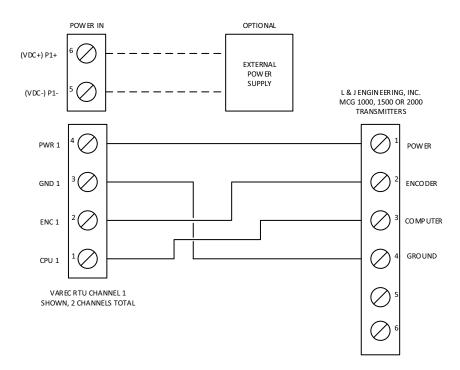
Figure 9–6: 8816 Tankway Module Field Wiring
