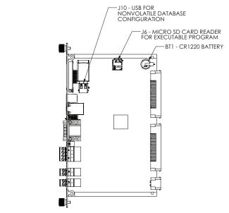
*Figure 4–2: 8811 CPU Module Side View*
