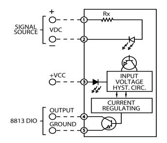
*Figure 6–3: 8813 Digital DC Input Solid–state Relay*
