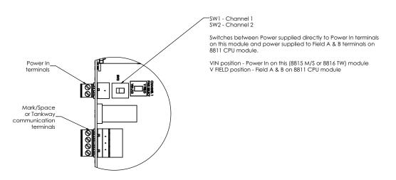
*Figure 8–3: 8815 Mark/Space Module Terminals and Switches Closeup*
