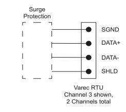
Figure 4-3: 8811 CPU RS-485 Terminals Connection
