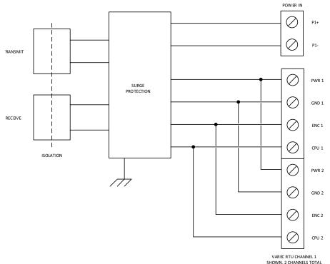
A schematic illustrating the terminal connections of the 8816 Tankway module is shown below:
