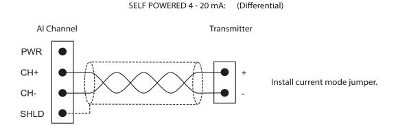
Figure 11–7: 8818 Analog Self–Powered 4–20 mA (Differential) Wiring
