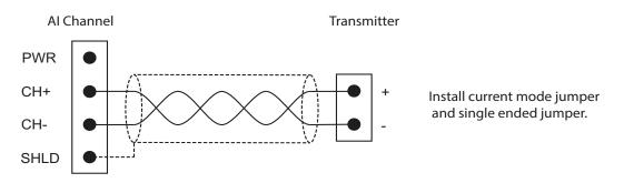
Figure 11-6: 8818 Analog Self-Powered 4-20 mA (Single Ended) Wiring
