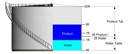
Example 1 shows how the product and water volumes are calculated when the water level is less than the water table
