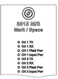
Figure 8-4: 8815 Mark/Space Module LED Indicators
