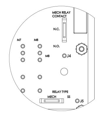
Figure 6-10: 8813 Digital Input/Output Module Watchdog Switch Details
