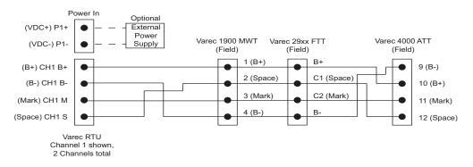
Figure 8–6: 8815 Mark/Space Module Field Wiring
