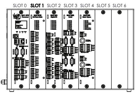
Figure 5-1: 8810 RTU with the 8812 Bi-Phase Mark Module in Slot 1
