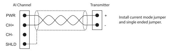
Figure 11-5: 8818 Analog Loop Powered 4-20 mA Wiring
