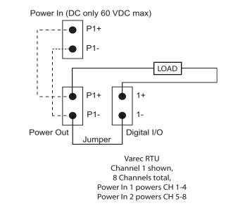
Figure 6-7: 8813 DC Output Wiring Diagram – RTU Powered
