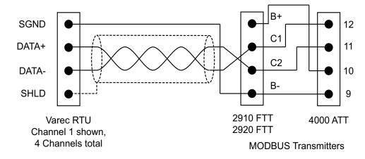
Figure 7-5: 8814 Serial Module RS-485 Field Wiring
