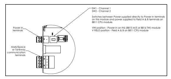
Figure 9-4: 8816 Tankway Module Terminals and Switches Closeup
