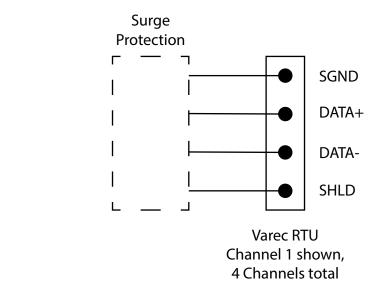
Figure 7-4: 8814 Serial Module RS-485 Terminals
