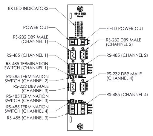
Figure 7–1: 8814 Serial Module Front View
