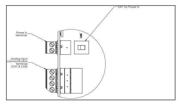
*Figure 11–4: 8818 Analog Input Module Terminals and Switch Closeup*
