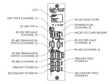
Figure 4-1: 8811 CPU Module Face Place
