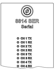
*Figure 7–3: 8814 Serial Module LED Indicators*
