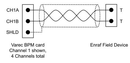
Figure 5-5: 8812 Bi-Phase Mark Field Wiring
