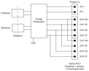
Figure 8-5: 8815 Mark/Space Module Terminals
