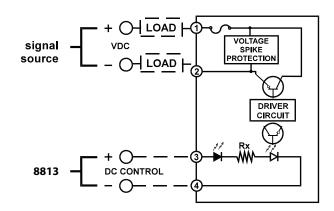
Figure 6-6: 8813 Digital DC Output Solid-state Relay
