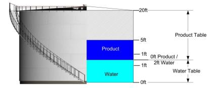
This example shows how the product and water volumes are calculated when the water level is equal to the top point in the water table.
