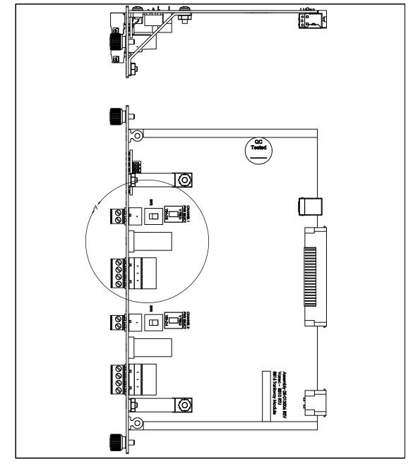
Figure 9-2: 8816 TW Tankway Module Top and Side Circuit Boards
