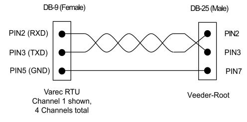
The following diagram shows how to use the 8814 Serial Module with Veeder-Root Modbus devices such as the TLS-3xx gauge line.
