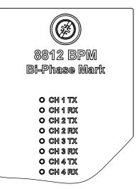
*Figure 5–3: 8812 Bi–Phase Mark Module LED Indicators*
